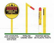
Natural gas is non-toxic, colorless, odorless and combustible. For detection and safety, the Natural Gas Division ensures the natural gas in Susanville has an unpleasant odorant called Mercaptan, (smells like rotten eggs) added to the natural gas traveling through its pipelines. For a "scratch and sniff" sample call 530-257-1041. Visible signs of a possible leak are provided below.
