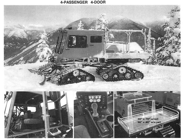
ENGINE ...... QSB 130 H.P. Tier 4 Final Cummins Diesel
